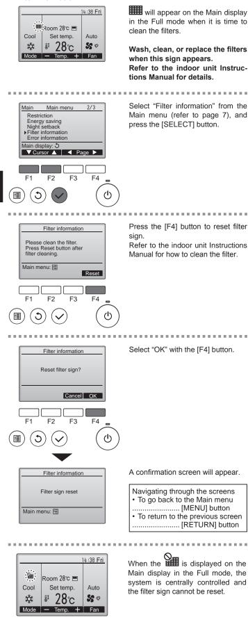
If two or more indoor units are connected, filter cleaning timing for each unit may be different, depending on the filter type.
